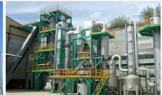
Wood chips Gasifier Plant 1.6 MWe CHP. Valencia, España
